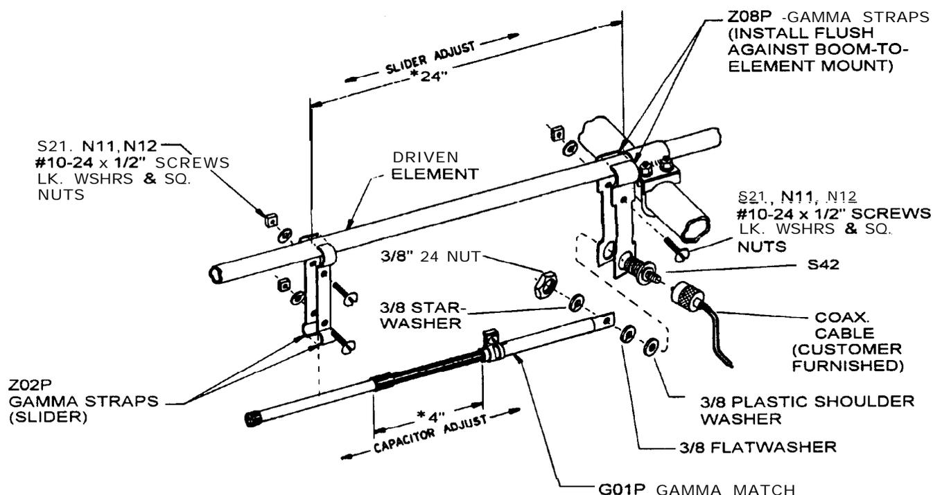
**FIGURE 4** GAMMA MATCH MOUNTING
